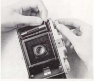
Turn the WINDING KNOB anti-clockwise and draw it outwards. Put the empty spool in this recess, slipping one end on to the bearing pin
