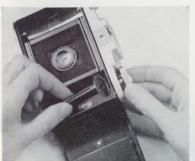
Check whether the FILM REMINDER is set for the film you are going to use. Only when the spool release knob is out can the reminder disc be turned to bring the name of the film against the diamond pointer on the top of the camera.
