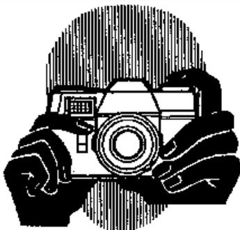
For horizontal shots hold the camera firmly with the right hand, with the index finger resting lightly on the release key. The second and third fingers of the left hand can be used to turn the focusing ring.
